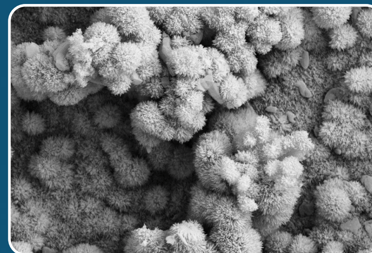
▲ Calcium phosphate precipitated crystals scattered on the hydrated tricalcium silicate cement surface.
